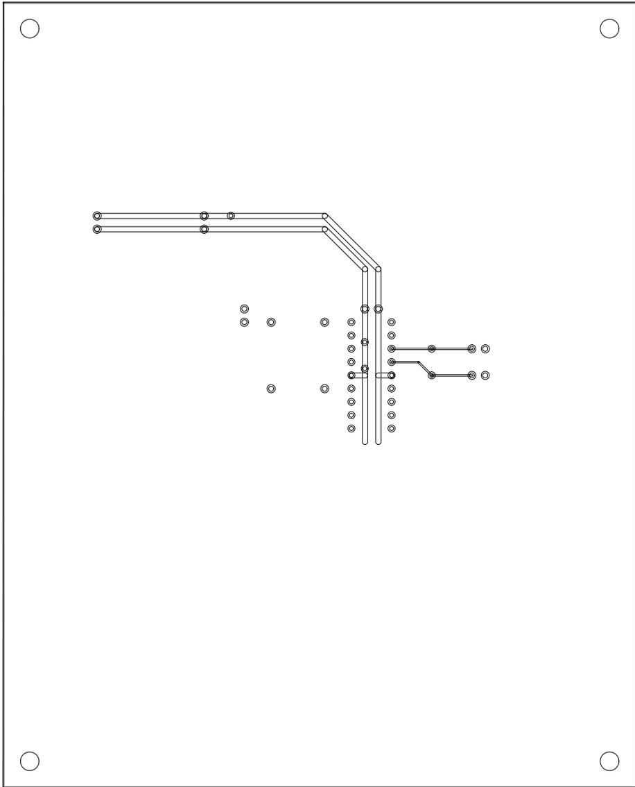
24 : Solider Side Pattern Sample Circuit
